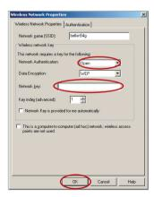
**Important:** A WEP key is a mixture of numbers and letters from A–F and 0–9. For 128-bit WEP, you need to enter 26 characters. For 64-bit WEP, you need to enter 10 characters. This Network key needs to match the key you assign to your Wireless Modem/Router or access point.
